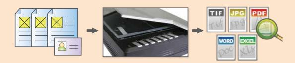
Industry standard TWAIN and WIA drivers combined with TIFF, JPG, PDF and Microsoft Office file formats ensure compatibility with thousands of scanning and imaging programs. Built in Plustek OCR (Powered by ABBYY® FineReader®) allows you to convert files into editable and searchable.
